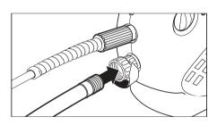
→ STEP 4: Connect garden hose to the cold water source and turn water on completely. Plug the power cord into the power outlet.
